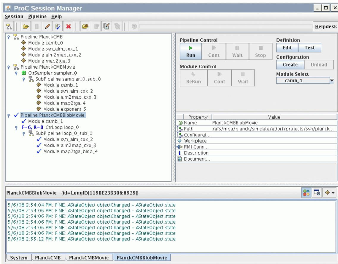
**Fig. 2:** The GUI of the Planck Process Coordinator (ProC) workflow engine. The ProC is mainly used within the Planck Surveyor project, but may be used for organizing the execution of other scientific tasks, including simulations and data analysis.
